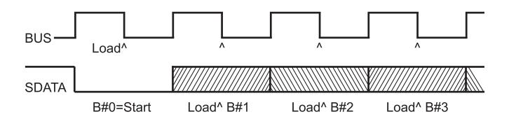
The data is latched into the internal shift register on the falling edge of the BCLK signal with the BCLK as a reference (see waveform above). The SDATA input pattern will change at the BCLK rising edges and must be stable for loading into the shift register at the BCLK falling edges.
