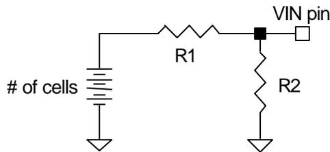
Figure 11: Resistor divider network at the VIN pin
