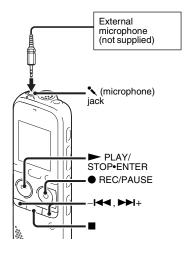
When you connect a stereo microphone (not supplied) to the IC recorder and the recording mode is set to "SHQ" or "HQ" mode, you can record sound in stereo.
