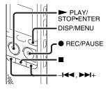
When "Add/Overwrite" in the menu is set to "Overwrite," you can add an overwrite recording after a selected point in a recorded file. The part of the file after the selected point is erased. The starting point of an overwrite recording
