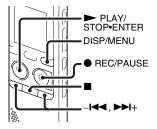
When "Add/Overwrite" in the menu is set to "Add," you can add a recording to the file being played back. The added recording will be placed after the current file, and will be counted as a part of the file.
