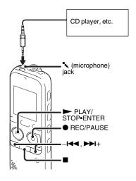
You can make music files without using the computer by recording sound from other equipment connected to the IC recorder. When you select "Audio IN" in the "Scene Select" menu, the settings suitable for recording from other equipment are already selected. For details on setting, see page 30.
