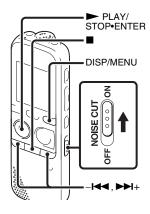
When you slide the NOISE CUT switch to "ON" in the playback mode, ambient noise other than the human voice is reduced. A file is played back with clear sound quality because the noise of all frequency bands including a human voice is reduced.
