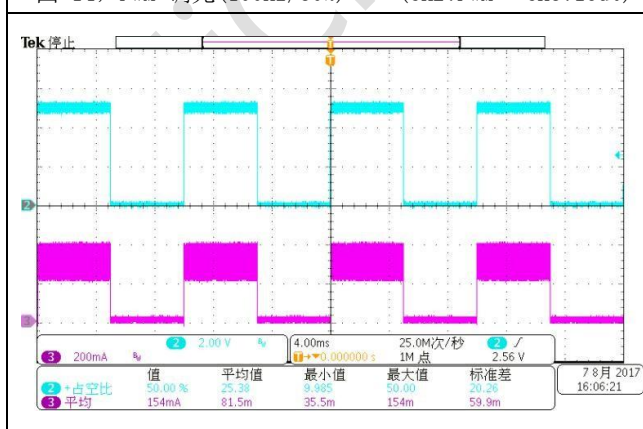
图 14, PWM 调光 (100Hz/50%) (CH2:PWM CH3:Iout)
