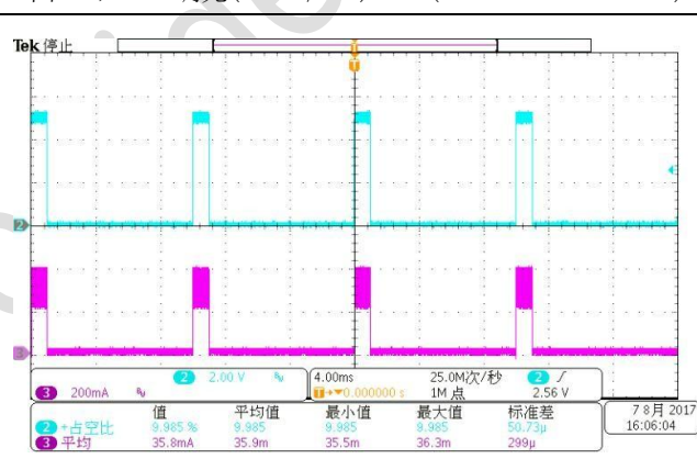
图 13, PWM 调光 (100Hz/10%) (CH2:PWM CH3:Iout)
