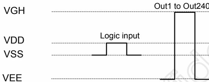
The input signal level of CPV, L/R, OE, STV1, /XAO and STV2 have to swing between VDD and VSS. The signal output level of start pulse (STV1 or STV2) to the next stage cascaded device is VDD for H and VSS for L.
