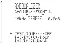
Use this feature to make adjustments of “GEQ” while listening to a test tone. To select “TEST TONE”, press ▼ repeatedly in the graphic equalizer screen.
