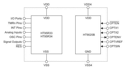
Internal Chip Interconnection Diagram
