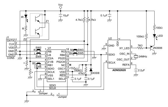
Note: \* For resistor value selection, refer to high or low input level of Z1 and Z2 in the D.C. Characteristics table. The recommended value is  $6k\Omega$ .
