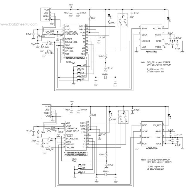
Note: Place the  $0.1\mu$ F capacitor,  $22\Omega$  resistor and  $0.01\mu$ F capacitor as close to VDD pin as possible.
