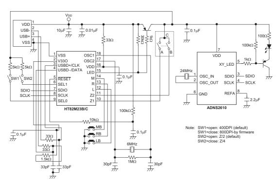
Note: Layout  $0.1\mu F$  capacitor,  $33\Omega$  resistor and  $0.01\mu F$  capacitor as close to VDD pin as possible.
