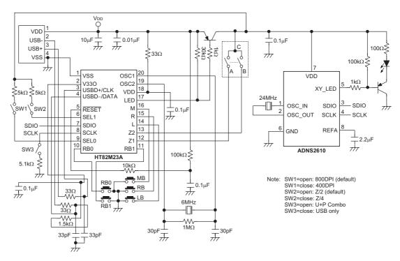
Note: Layout  $0.1\mu\text{F}$  capacitor,  $33\Omega$  resistor and  $0.01\mu\text{F}$  capacitor as close to VDD pin as possible.
