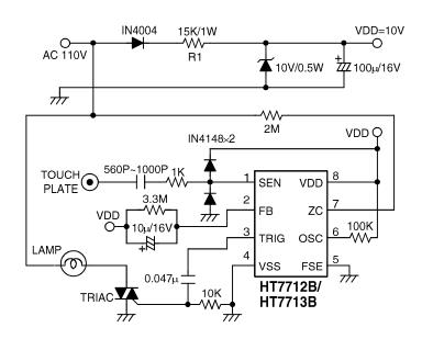
Note: 1. In 220V AC line power, the R1=33K/1W
