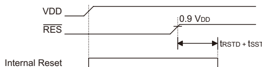
Power-on Reset Timing Chart
