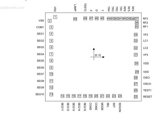
Chip size:  $2680 \times 2460 \ (\mu m)^2$ Chip thickness=12 mil
