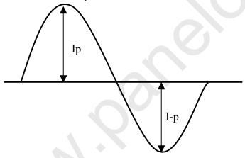
Asymmetry rate =  $|I_p-I_{-p}| / I_{rms} \times 100\%$ Distortion rate =  $I_p$  (or  $I_{-p}$ ) /  $I_{rms}$
