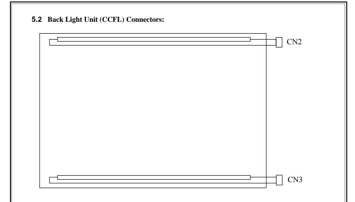
CN2, 3: CCFL Power Source (BHR-03VS-1/Japan Solderless Terminal MFG Co., LTD) Mating connector: SM02 (8.0)B-BHS-1/ Japan Solderless Terminal MFG Co., LTD
