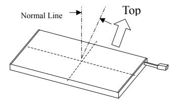
**Note (7)** Measurement at the center area of the panel when all the input terminals of LCD panel are electrically opened
