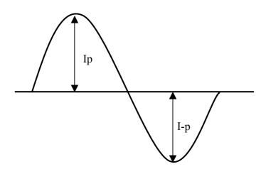
Asymmetry rate =  $|I_p-I_{-p}| / I_{rms} \times 100\%$ Distortion rate =  $I_p$  (or  $I_{-p}$ ) /  $I_{rms}$
