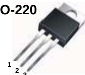
1.Gate 2. Drain 3. Source
