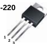
1.Gate 2. Drain 3. Source
