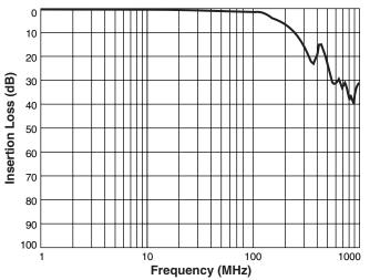
802.3af specification: 1.0 min dB from 0.1 MHz to 100 MHz 1.2 min dB at 125 MHz
