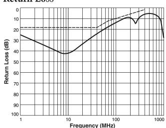
802.3af specification: 18 dB min from 1 MHz to 40 MHz 16 dB min at 50 MHz 12 dB min at 80 MHz 10 dB min at 100 MHz
