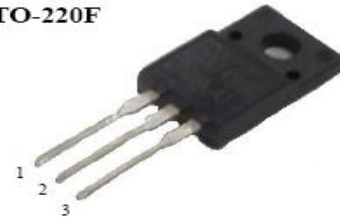
1. Gate 2. Drain 3. Source
