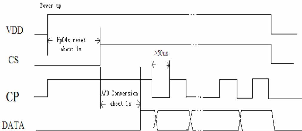
After finish ADC, DATA pin would change from low level to high level, once control system detect DATA is high level, then it send Clock for data.
