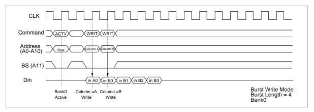
**Same bank, different ROW address:** When the ROW address changes, consecutive write commands cannot be executed; it is necessary to separate the two write commands with a precharge command and a bank-active command.
