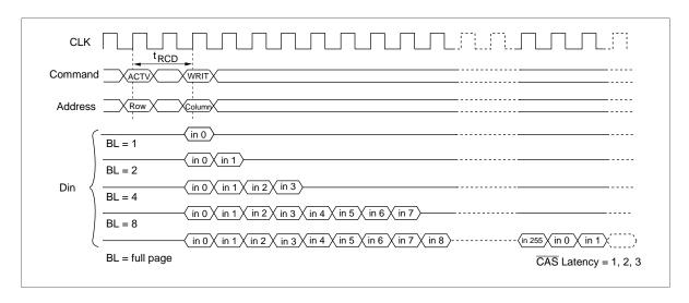
**Single write:** A single write operation is enabled by setting OPCODE (A9, A8) to (1, 0). In a single write operation, data is only written to the column address (AY0 to AY8; HM5216805 Series, AY0 to AY9; HM5216405 Series) and the bank select address (A11) specified by the write command set cycle without regard to the burst length setting. (The latency of data input is 0).
