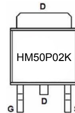
Marking and pin Assignment
