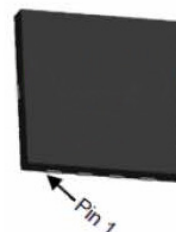
DFN 3.3x3.3 EP top view
