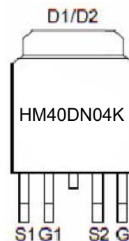
Marking and pin assignment
