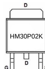
Marking and pin Assignment
