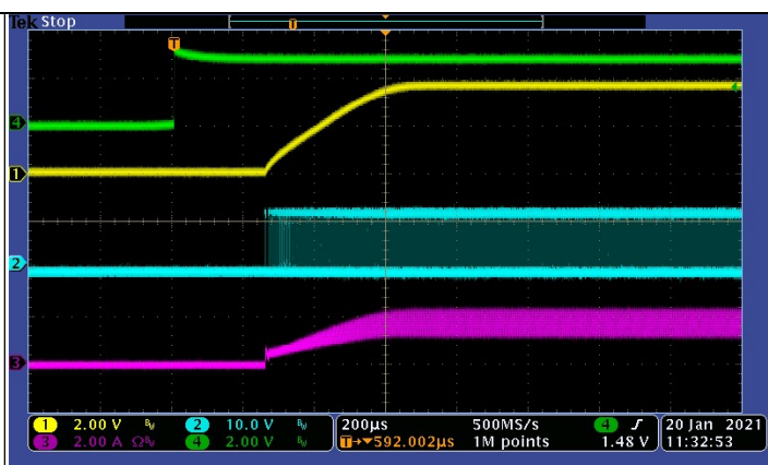
Fig 8 Enable Start up ( V_{in}=12V , V_{out}=3.3V , I_{LOAD}=2A )
