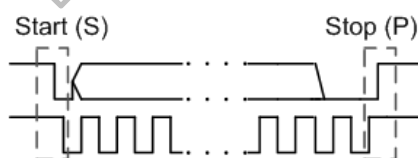
Figure 8.1: 2-Wire serial interface Start / Stop condition
