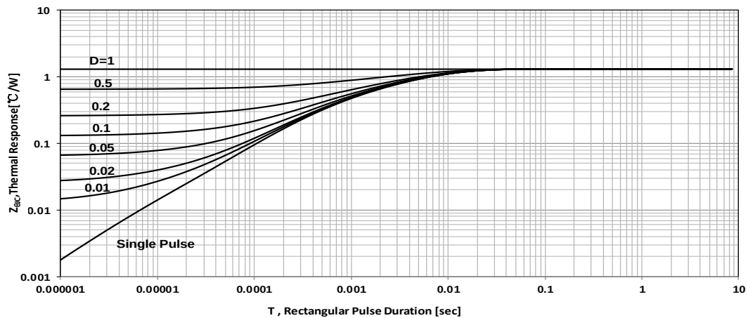
Figure 5 Maximum Effective Thermal Impedance , Junction to Case
