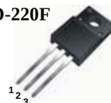
1.Gate 2. Drain 3. Source
