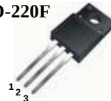
1.Gate 2. Drain 3. Source
