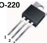
1.Gate 2. Drain 3. Source
