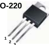
1.Gate 2. Drain 3. Source
