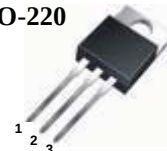
1. Gate 2. Drain 3. Source
