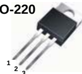
1.Gate 2. Drain 3. Source
