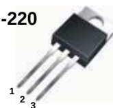
1.Gate 2. Drain 3. Source
