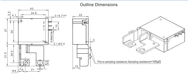
Remark: 1) The dimension of the load terminals as well as the sampling resistance can be made per customer request.
