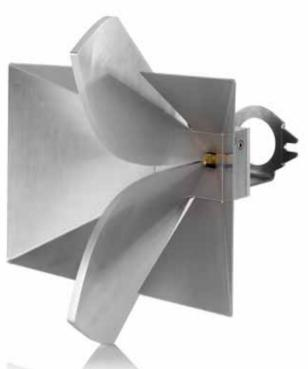
The linearly polarized R&S®HF907 double-ridged wave-guide horn antenna is a broadband, compact transmitting and receiving antenna for the frequency range from 800 MHz to 18 GHz.
