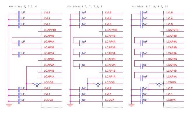
Different duties require different bias settings. There is some reference correspondence between the Duty and Bias Setting. However, it is better to use it as starting point and adjust it with real LCD panel connected to it to determine the final setting. The relationship between the duty and bias setting is just for reference as following:
