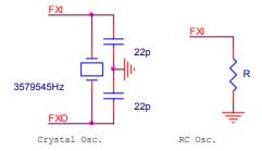
The RC oscillator has a built-in capacitor. An external resistor is needed to connect from FXI to GND to determine the oscillation frequency. The capacitance of internal RC oscillator is selected by mask option MO\_RCAP[2..0].
