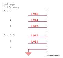
For example, if the bias setting is 1/7 bias and LVL2 is 2 volts, the LVL5 will be pumped to 7 volts when the load is light.
