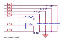
With the regulated LCD power, the LCD display can give steady visual effect over a wide range of operating voltage. The built-in regulator must be enabled by mask option MO\_LVRG to function.
