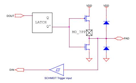
PRT11[7..0], PRT14[7..0], PRT15[7..0] and PRT17[7..0] share pads with SEG[8..39]. The function of the pins is selected by mask option MO\_LIO11, MO\_LIO14, MO\_LIO15, MO\_LIO17 respectively as shown in the following figure.
