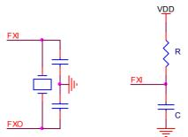
Two types of oscillator, crystal and RC, can be used as slow clock by mask option MO\_SXTAL. If used in for time keeping function or other applications that required the accurate timing, crystal oscillator is recommended. If the timing accuracy is not important, then RC type oscillator can be used to reduce cost.
