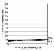
2.-(2) Electrical life test (High capacity type, Resistive load 250V AC, 48A at 85°C 185°F)
