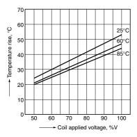
1.-(2) Coil temperature rise (High capacity type) Sample: HE1aN-P-DC9V-Y5, 6 pcs.
