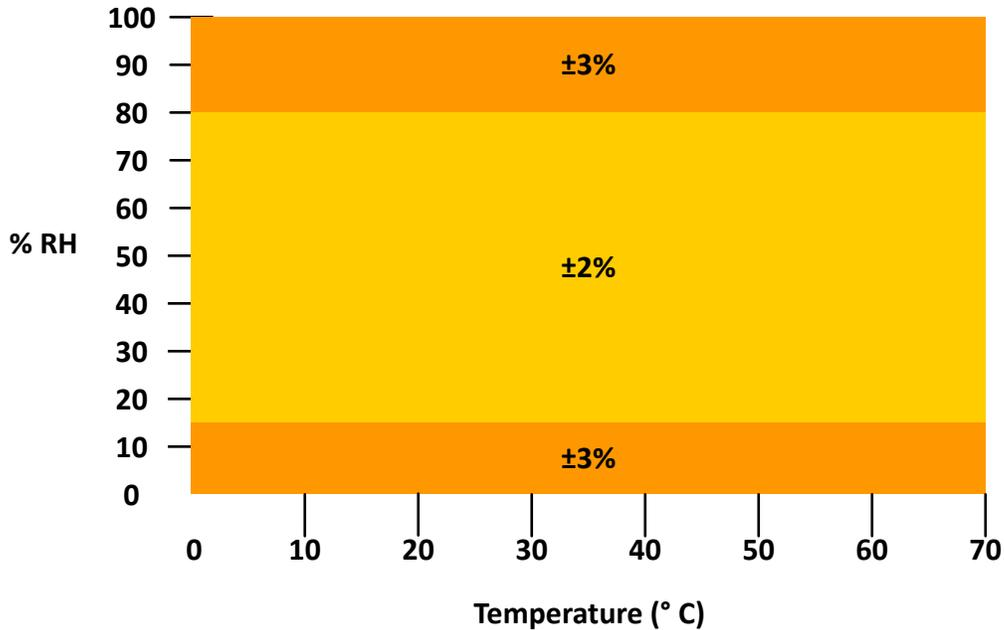
**Figure 11-1. Typical Relative Humidity Accuracy Range Limits**
