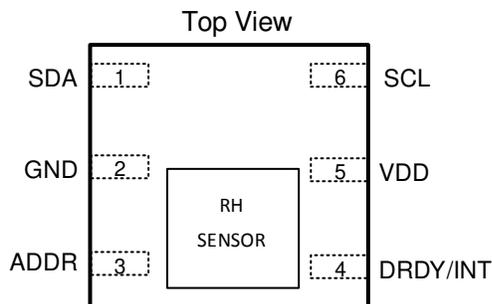
**Figure 6-1. DMB Package 6-Pin PWSON Top View**
