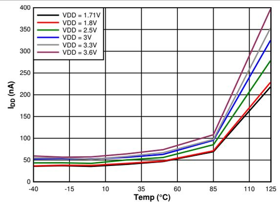
Figure 7-7. Supply Current vs. Temperature, Sleep Mode
