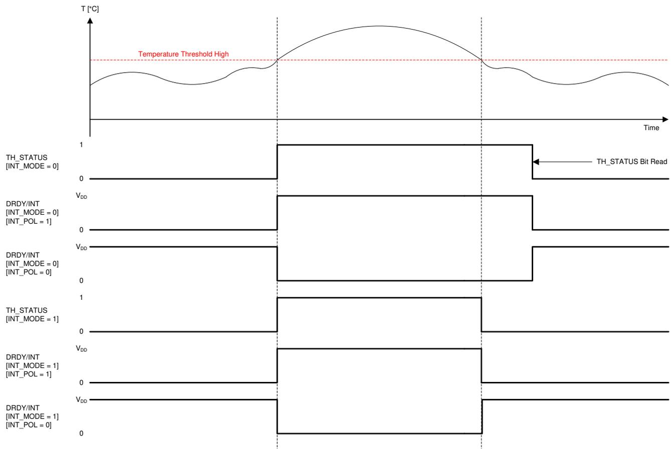
Figure 8-3. INTERRUPT on Threshold - Temperature High
