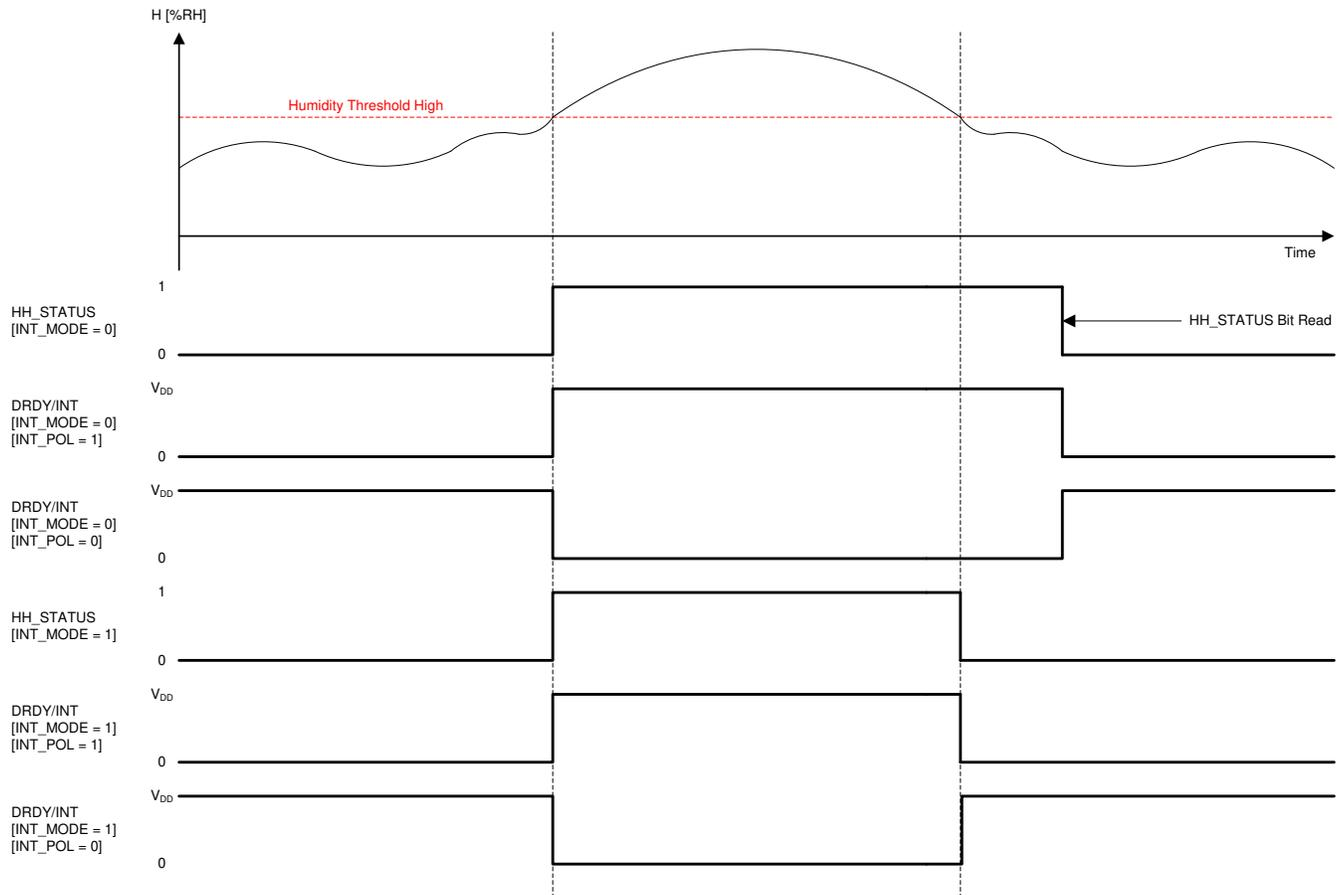
**Figure 8-5. INTERRUPT on Threshold - Humidity High**
