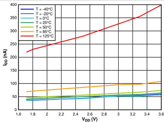
Figure 7-6. Supply Current vs. Supply Voltage, Sleep Mode
