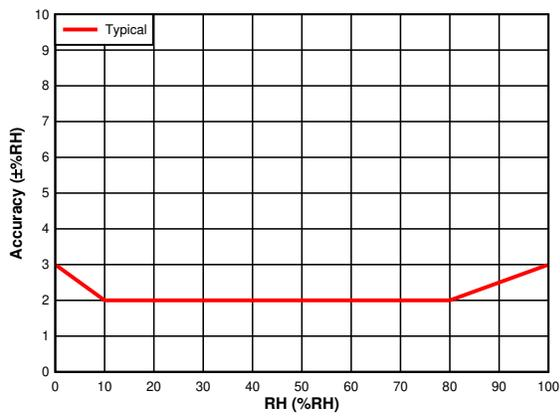
Figure 7-2. RH Accuracy vs. RH Set Point
