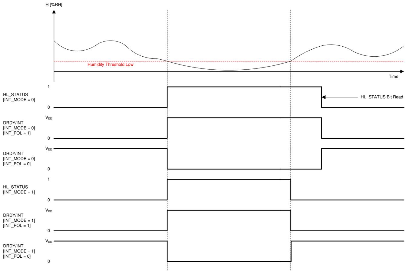
Figure 8-6. INTERRUPT on Threshold - Humidity Low
