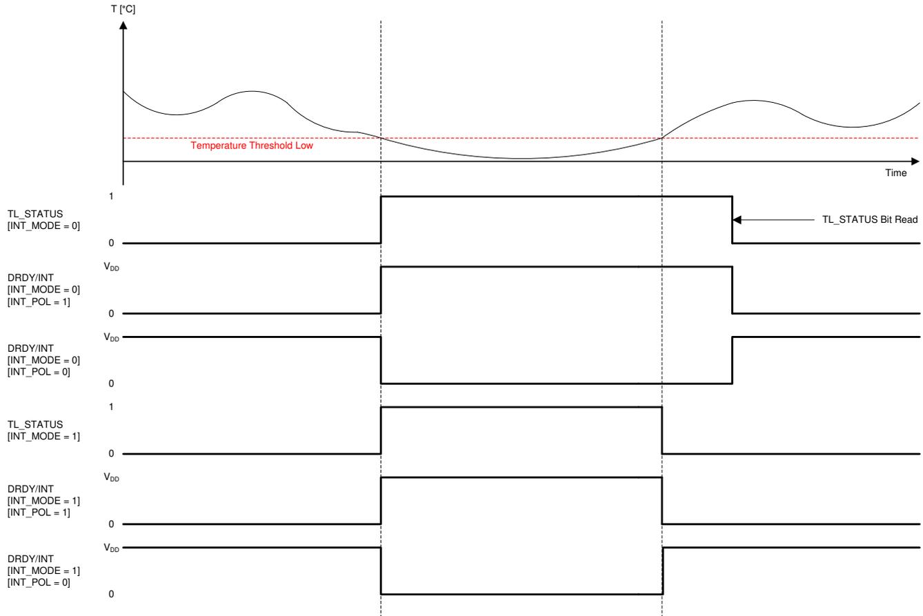
**Figure 8-4. INTERRUPT on Threshold - Temperature Low**
