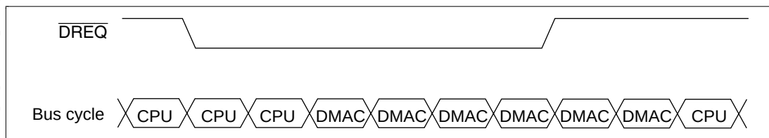
Figure 11.13 DMA Transfer Example in the Burst Mode
