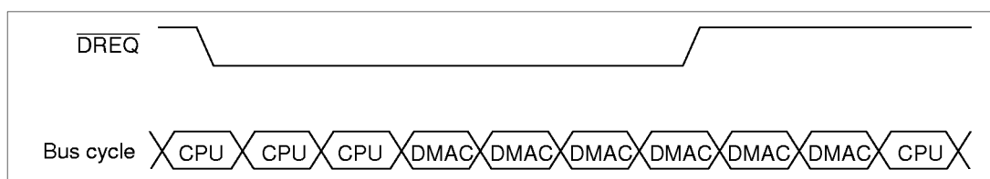
Figure 9.11 Transfer Example in Burst Mode (Single Address Mode, \overline{\text{DREQ}} Level Detection)
