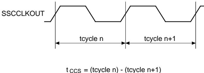
**Figure 1** Cycle to cycle jitter (SSCCLKOUT)
