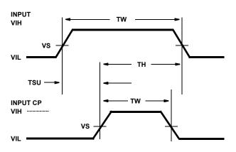
TH = HOLD TIME TSU = SETUP TIME TW = PULSE WIDTH
