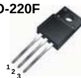
1.Gate 2. Drain 3. Source
