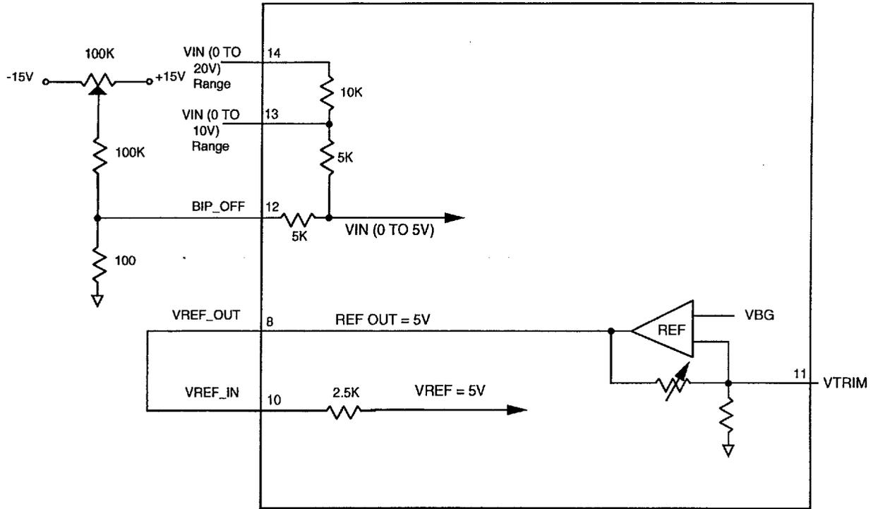
Note: If no offset adjustment is required, BIP\_OFF can be tied directly to AGND (0 volts).
