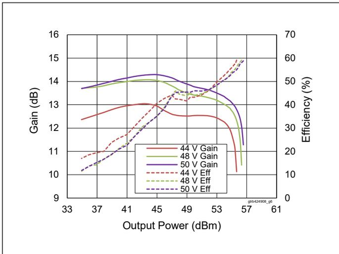
Figure 5. Pulsed CW Performance at Various  $V_{DD}$
