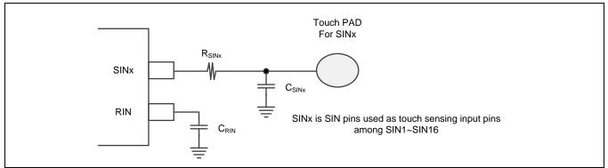
Implementation circuit for SIN pins and RIN pin is shown in the following figure.
